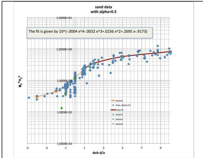
The curve for the case of buried charges defined above for  $d/a > 1$  is shown. In addition, the data and a fit for the near surface and height of burst data is also shown, with a polynomial fit to its log. That is the programed  $dob$  fit for all materials.
